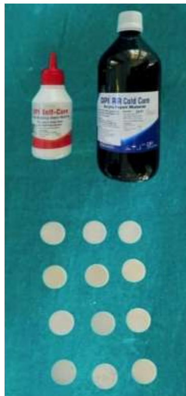
Figure 7 : Specimens After Immersion In Chlorhexidine And Octenidine Mouthrinses For 24 Hours
