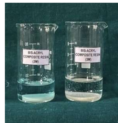
Figure 3. Immersion of specimen in Chlorhexidine and Octenidine mouthwash
