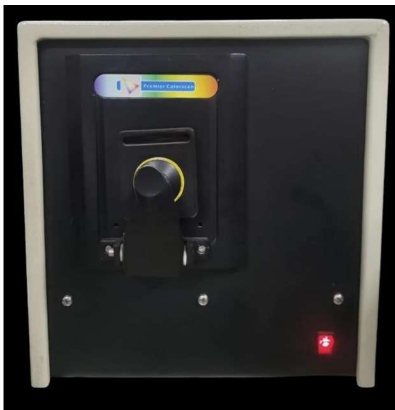
Figure 6: Premier Colorscan reflectance spectrophotometer (Premier Instruments, Mumbai, India) used for CIE L^*a^*b^* colour co-ordinate measurement under D65 illumination.
