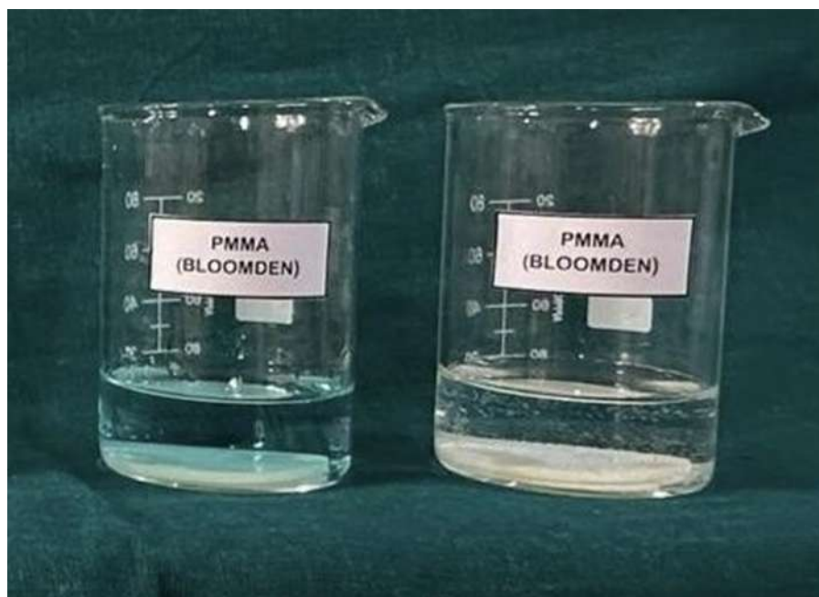
Figure 5: Bloomden PMMA disc specimens submerged in mouthrinses during the immersion protocol. Specimens were maintained at 37^{\circ}\text{C} \pm 1^{\circ}\text{C} throughout.
