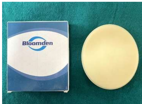
Figure 1: Bloomden CAD/CAM polymethyl methacrylate (PMMA) block (Vita shade A2; Bloomden Bioceramics Co., Ltd., China) used for specimen fabrication in the present study.
