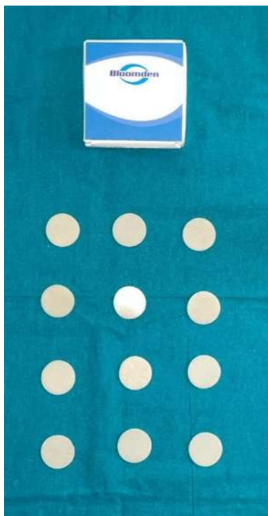
Figure 3: Twelve Bloomden PMMA disc specimens following standardised polishing and prior to allocation to experimental groups and immersion in mouthrinses.
