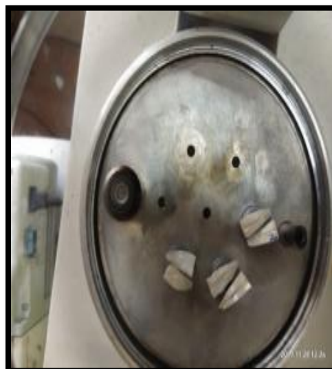
Figure 2 : Placement of sample on metal stud
