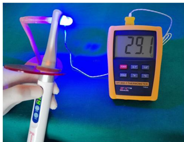
Figure 4: Application of LED light and Temperature measurement after applying bleaching agent
